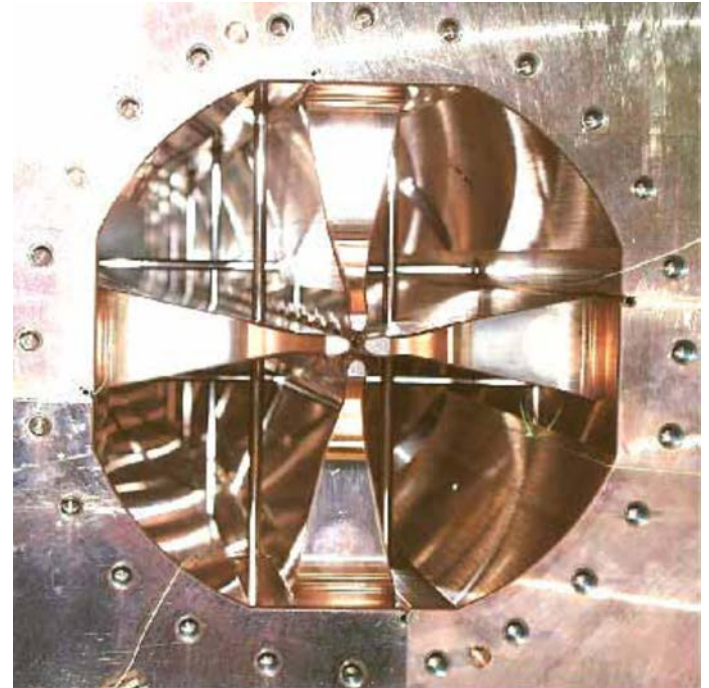
Inside view of RFQ
